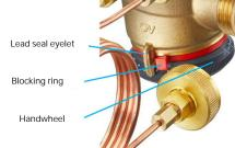
The nominal value setting is secured against unintentional setting by engaging the handwheel and the additional retractable blocking ring which can be fixed with sealing wire (item no. 1089091). The handwheel is always accessible and readable, even with the actuator mounted.
