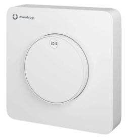
The ClimaCon F room thermostats are used to control the temperature of surface heating and cooling systems as well as heating and cooling ceilings in detached houses or flats. The room temperature is controlled via a valve, which is controlled by the room thermostat via an electrothermal actuator. When the room temperature reaches the target temperature, the valve is closed.
